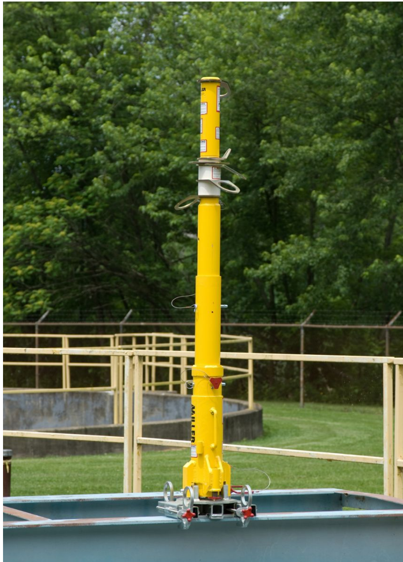
Figure 21: Three persons may be tied off to the post system for fall arrest at any given time. Adding extension or davit arm assemblies to the post reduces the capacity (Miller DuraHoist Portable Fall Arrest Post and Extension Post www.safety.honeywell.com ).
