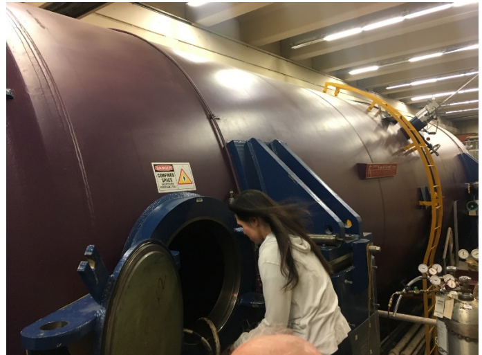
Permit-required confined space: Part of Van de Graaff accelerator used in nuclear physics and astrophysics research
