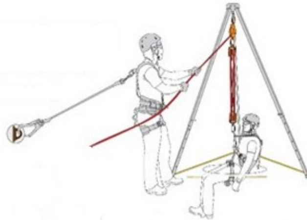
Figure 25: Attendant tied off for fall protection
