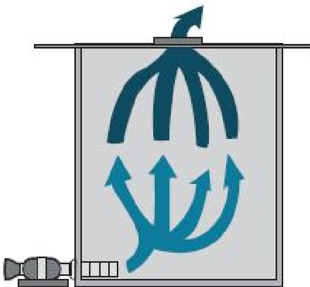
Figure 9: Blower positioned at the bottom of the space is blowing fresh air into the space and exhausting contaminants out the top opening. Source: www.ehsdb.com
