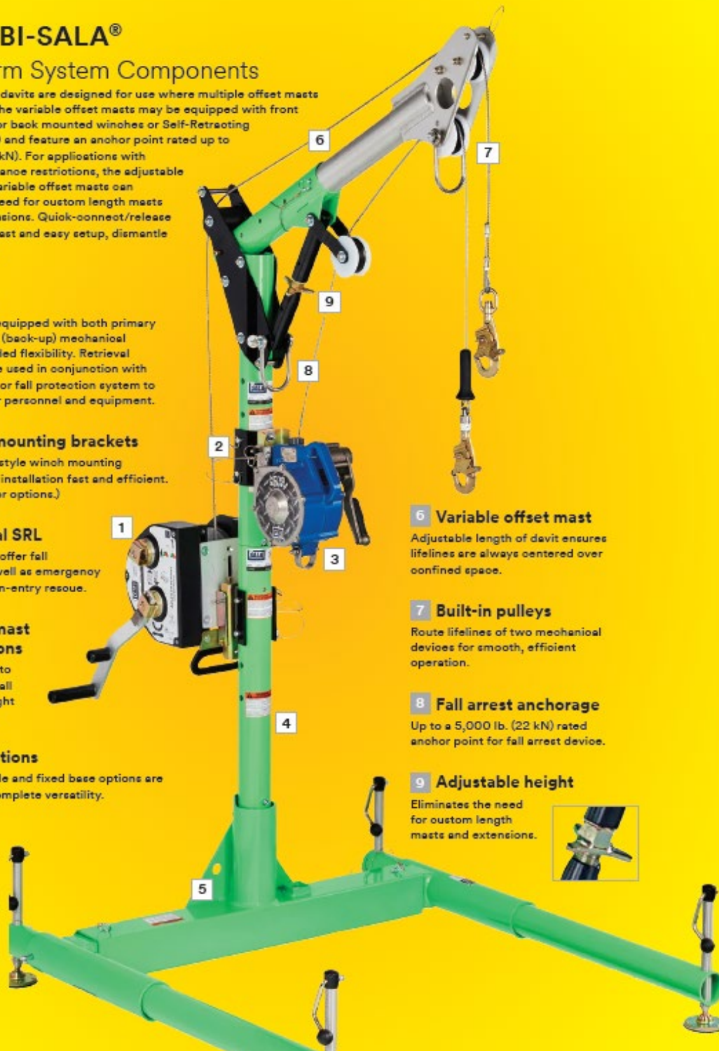
Figure 20: A davit arm prepared to provide fall protection and non-entry rescue. Designed to be mobile or permanently installed and can support vertical or horizontal entries (3M Company www.3m.com ).
