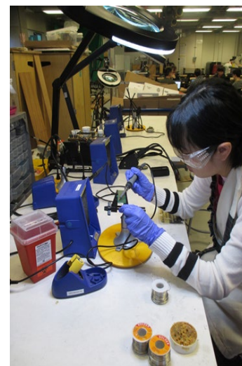
Designated soldering area with fume extractors at each station
