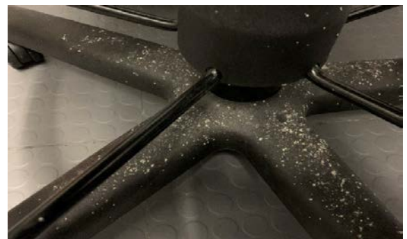
Mold growth on base of chair in cold room
