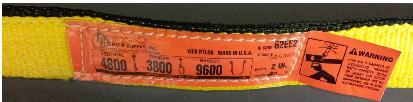
Figure 15: Nylon sling with load capacities for different rigging configurations (terranova.co.uk)
