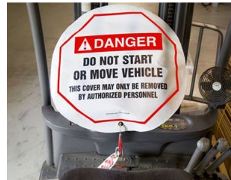
Forklift tagged out for service
